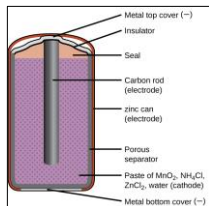
Figure 17.10: Dry Cell (or Laclanche) Batteries: Zinc container (anode), Graphite rod (cathode), 1.5 V
