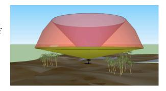
There are two main modes of operation for the Weather Service's Weather Surveillance Radar (WSR) 88D radars: Clear Air Mode and Precipitation Mode. Within these modes, forecasters can vary the number of elevation tilts and rotation speeds of the radar.
